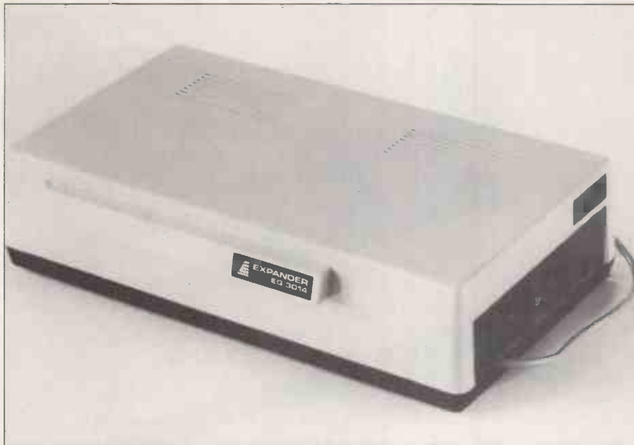
The expander box controls up to four disc drives and a printer.
